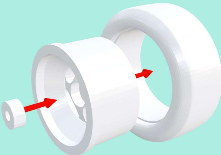
After assembling the wheels, these can easily be attached to the suspension.
