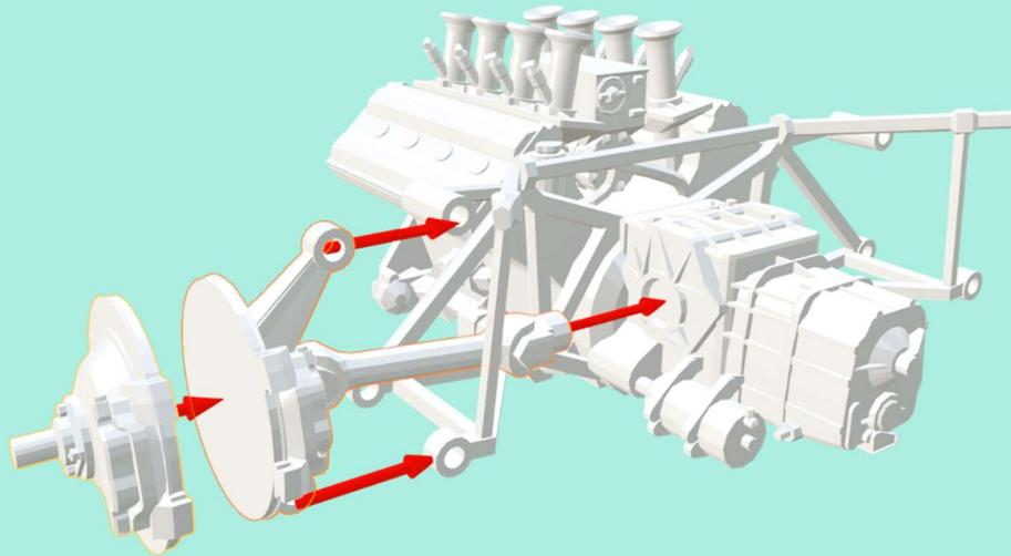
Now you can tighten these parts by attaching the engine mounting rods. Take care which rod goes where!
