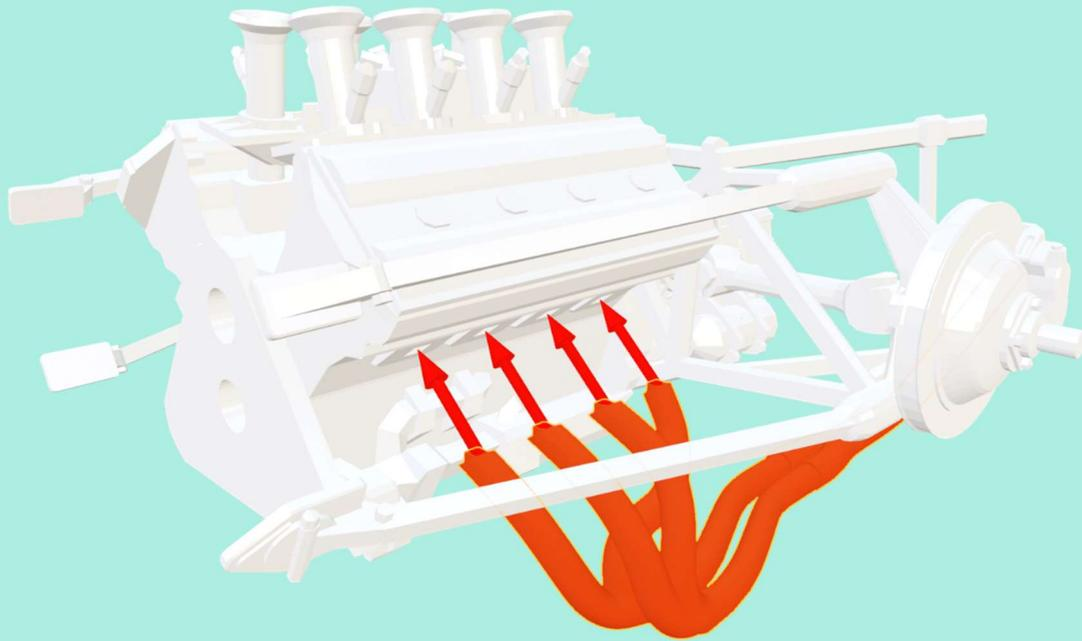
Fixate the exhaust pipes, using the bracket at the back of the gearbox, it should snap right on.
