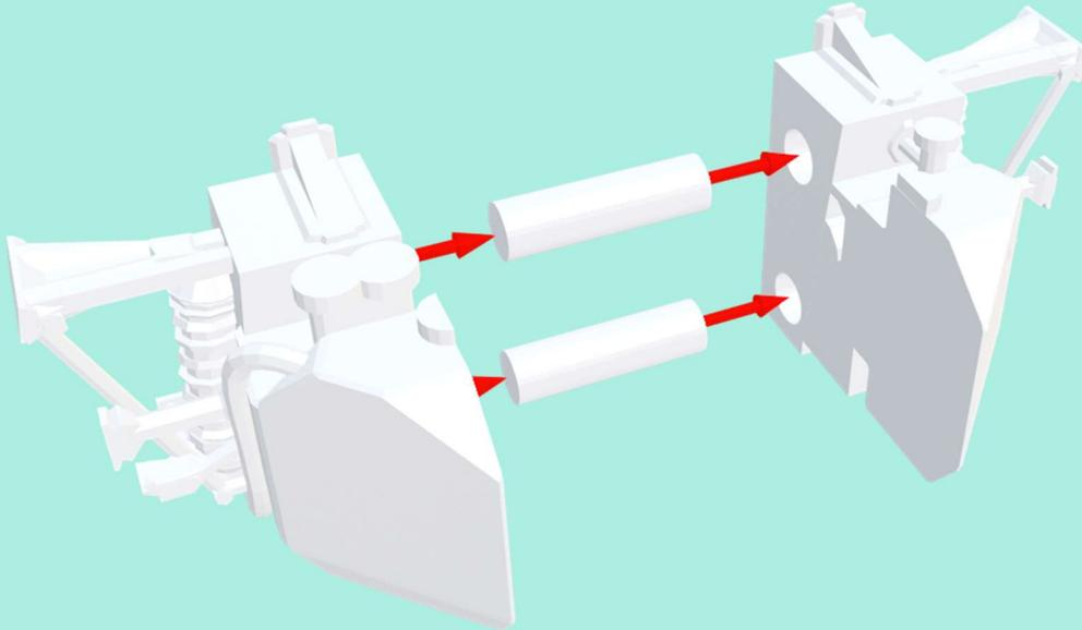
And proceed by connecting the front suspension arms and brake-disks.
