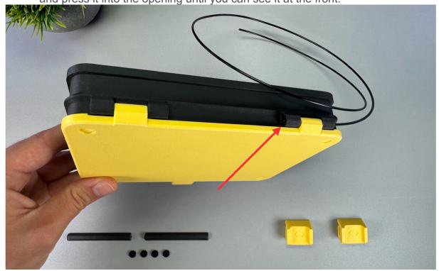
3. Cut the filament flush and do exactly the same on the other side
