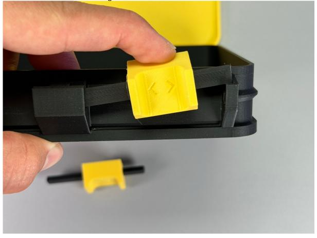
8. It must look like this! When the rail is to loose you can add a little bit of glue! Do this on the other side as well. Make sure that the two slide locks can be moved easily. If not, file away a bit.
